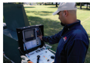
One of the new features of the PFL20M-1500 is the lid-mounted MTDR that offers multiple test modes and simple, easy pushbutton operation.
