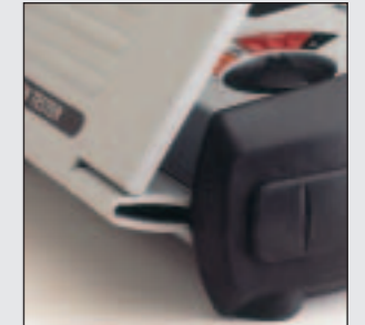
Double hinge keeps screen free from scratches or swings under to snap out of sight
