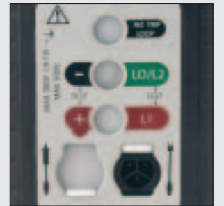
Test lead panel with interlock to prevent hazardous lead combinations
